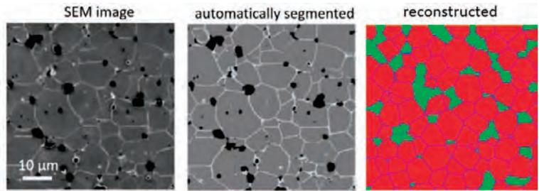
Fig. 2 Synthetic microstructure generation based on SEM images.
