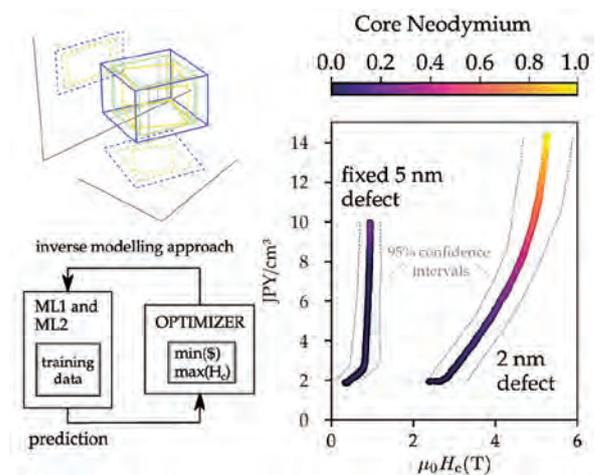
**Fig. 1** Minimizing materials costs and maximizing coercive field by multi-objective optimization using machine learning models (ML) as surrogate. ML1 predicts the intrinsic magnetic properties from the chemical composition; ML2 predicts the coercive field from the intrinsic properties and the geometry. The right part shows the Pareto fronts for a fixed soft magnetic defect thickness of 2 nm or 5 nm. The results show the Nd-content of the core can be reduced significantly.
