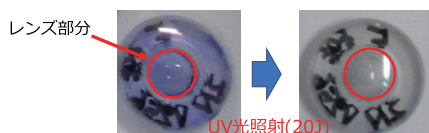
Fig. 3 Marker ink disappeared after UV radiation
