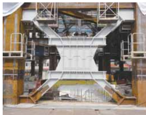
Fig. 1 Fe-15Mn-4Si-10Cr-8Ni alloy seismic damper [1].
